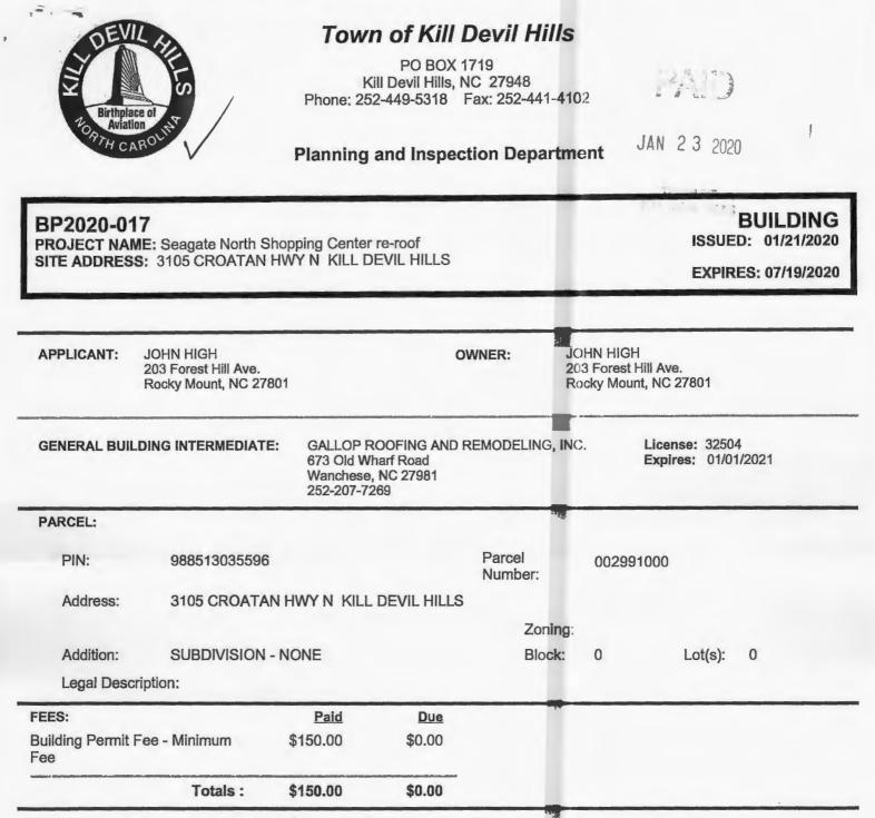
**PROJECT DESCRIPTION:** Remove and replace fully adhered 50 mil PVC roof w/ required peel stop strips.
