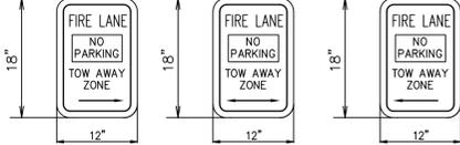
\* NO PARKING - FIRE LANE SIGNS SHALL BE PLACED ON BOTH SIDES OF THE ACCESS ROAD. (SEE DETAIL BELOW). SIGNS SHALL BE SPACED NO MORE THAN 100 FEET APART FROM EACH OTHER. SIGNS SHALL BE METAL, REFLECTIVE AND SHALL FACE THE FIRE LANE. SIGNS SHALL BE MOUNTED ON A POLE OR THE BUILDING, AT LEAST 5' BUT NOT MORE THAN 7' A.F.G.
