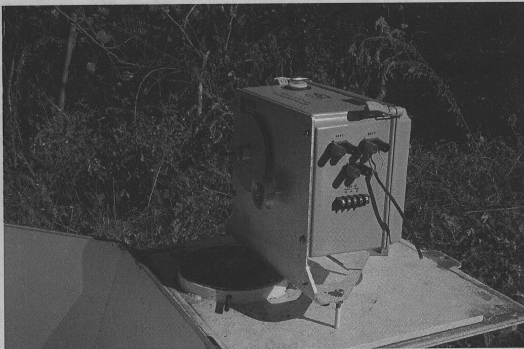
Figure 3: Sutron 8400A shaft encoder with integral data logger. Top picture shows front view of recorder. Bottom picture shows rear view with float and counterweight lines going into well.
